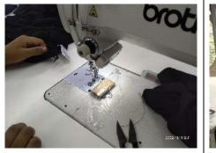
Needle guard was misplaced with sewing plain machine **NC Picture No.07**
